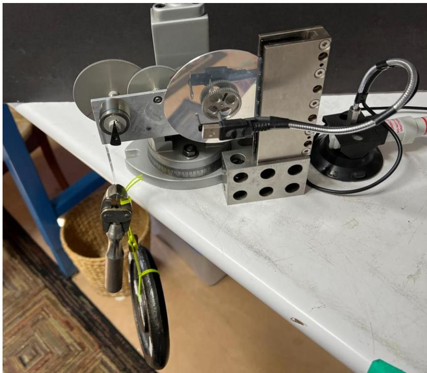
The drive method is a 1" mandrel added to Wheel 1, which uses a .003" thick stainless band spirally wrapped a few times, and a roughly 5.5 lb dead weight. The disadvantage of the band-wrap unwinding
